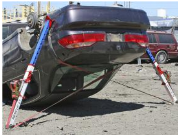
Chain saddle lifting
